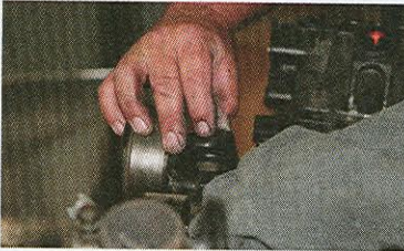
15. This is the largest of many O-rings in the gasket kit; it makes the seal between the manifold and one of the coolant passage tubes.
