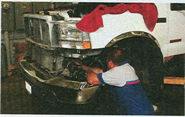
29. Now that the engine is largely done, it's time to lower the body closer to the chassis and think about making connections. It was necessary to slowly and carefully lower the cab, so as not to pinch or crush anything as it comes back together.
