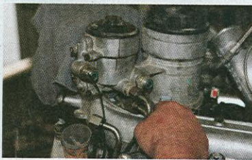
28. There are three lines connecting to the fuel filter, each requiring a new O-ring. Two lines feed fuel in; the third is a fuel return line.
