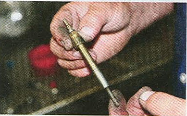
17. Glow plugs can now be installed.
