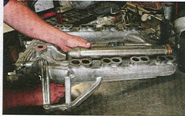
13. The EGR cooler can be positioned on the intake manifold now. This one is based on the newer Ford design. It was cleaned out in the solvent tank, removing a lot of soot and pressure tested before reinstallation.
