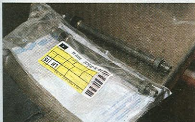
1. This is the standpipe for the high-pressure oil/fuel system. These are generally discarded upon disassembly and replaced with new parts.
