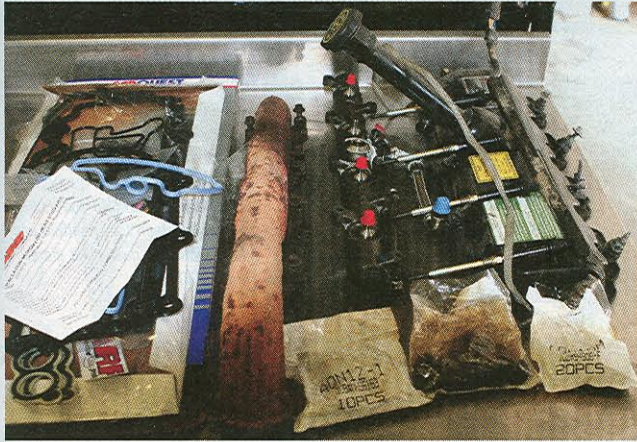
We still have an ugly pile of pieces kicking around, including the intake manifold, injectors and fuel rail, turbo, EGR cooling system, valve covers and a bunch of gaskets. This ain't the fun part, but they gotta go back on.
