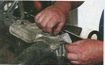
22. Don't forget the heat shield; otherwise the heat from the turbo can create a hot spot on the manifold.
