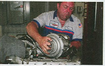
23. The original stock turbo, newly cleaned and balanced, goes back on the engine.
