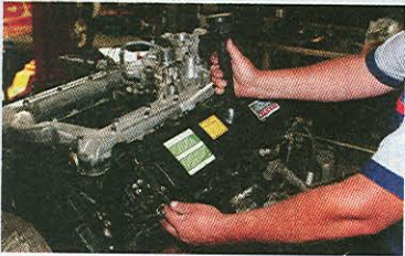
20. Then the valve cover itself can be installed.
