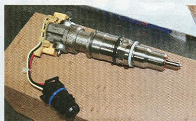
4. When the old injectors were found to be out of spec, eight new injectors were purchased.
