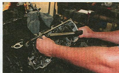
3. Tighten to spec (33 lb-ft).
