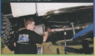
Matthews installed the 4-inch pipe by connecting it to the catalytic converter, where the new exhaust system starts.
