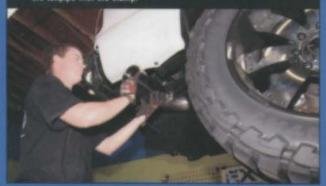
Matthews cut off approximately 3 inches of the tailpipe so the tip would not protrude from the truck as much as the clamped install. The shorter tallpipe gives the truck a cleaner look while still allowing the striking polished tip to be seen.
