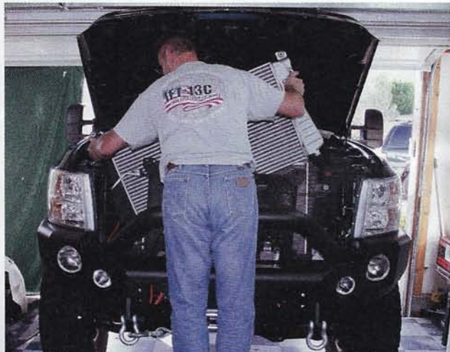
Finally, we unbolted and removed the stock intercooler from the truck.
