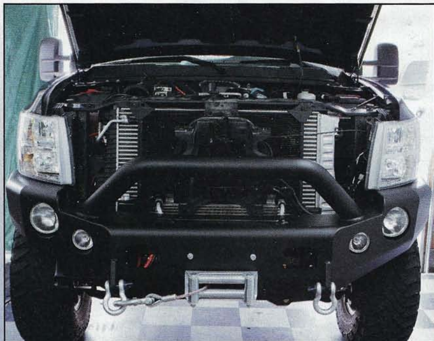
Next, the grille support braces and headlight mounts were removed.
