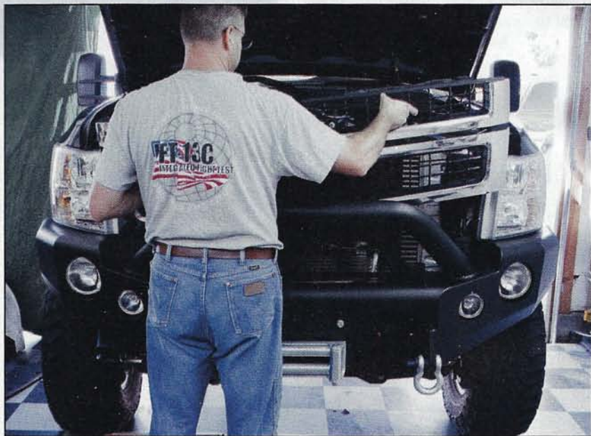
The process began by removing the grille and the Banks Ram-Air filter and mounting bracket.
