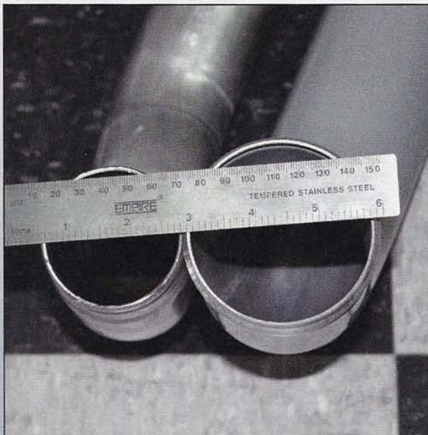
Size does matter. The banks tube (right) is 33 percent larger than the stock tube.
