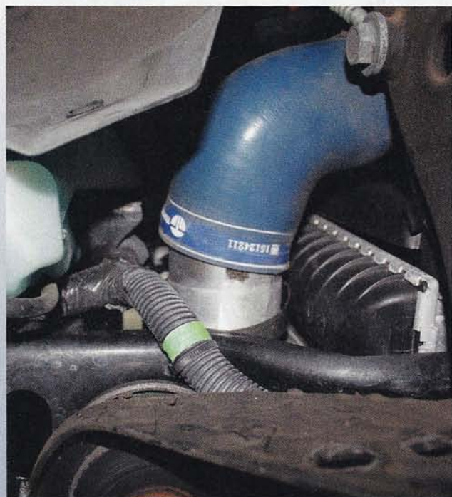
We then loosened the intercooler boost tube T-clamps and removed the elbow.
