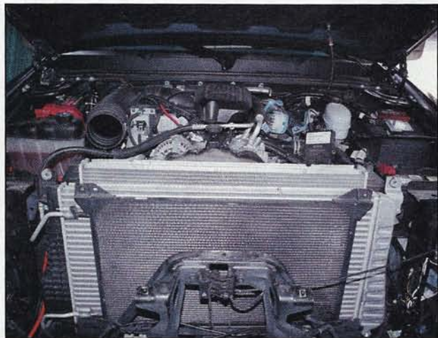
Then we removed the upper radiator support bracket.
