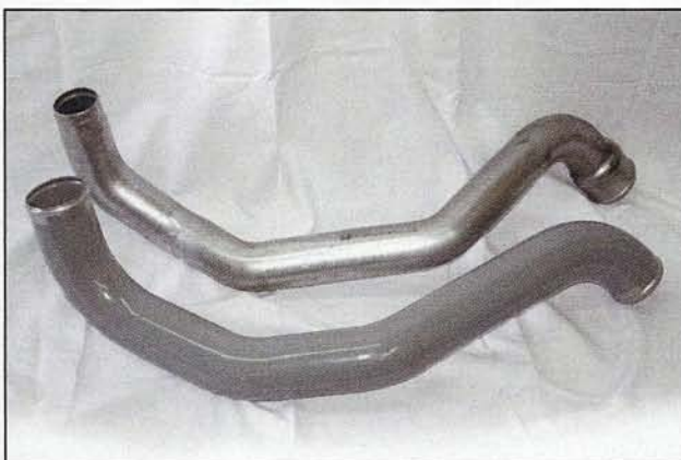
Here's a look at Banks' hot-side boost tube next to the OEM version. Notice the smooth mandrel-bends and high-quality powdercoating on the Banks tube.
