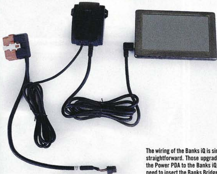
The Banks iQ includes a quick-release clip, windshield mount, Banks Bridge Module, OBDII interface connector, thermocouple cable, Y-cable, USB cable (mini B to USB), instruction manual, miscellaneous hardware, and a charger (not pictured).
