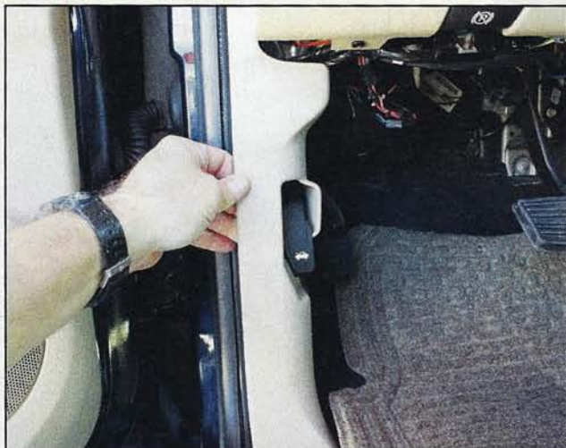
To make cable routing easier, we removed the driver-side kick panel by gently pulling on it to release the two spring clips.
