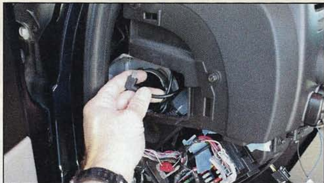
Only the USB power cable needs to be routed up to the Banks iQ. Removing the fuse box access panel made this an easy task.
