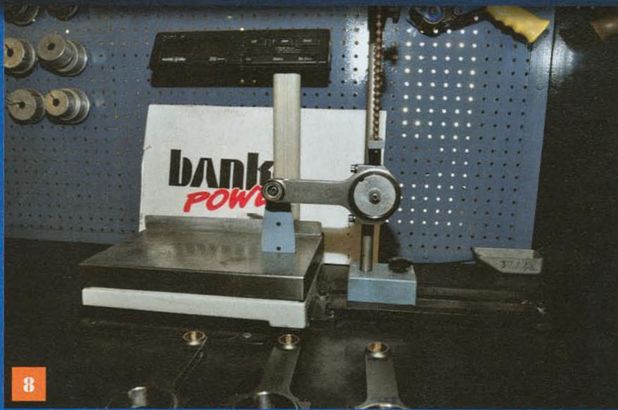
ABOVE: The connecting rods must be carefully weighed to within one gram of each other.
