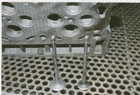
11. After 10 minutes of blasting away carbon, the heads and valves are clean as a whistle with a satin finish.
