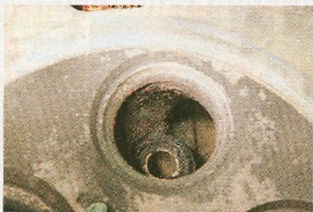
8. The exhaust ports were much worse, with clumps of crud accumulating inside.
