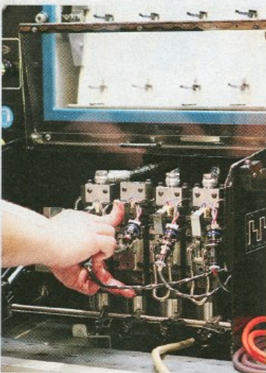
3. To test the injectors, they are attached to a Hartridge HA 230 injector tester at BECS in Whittier, CA.
