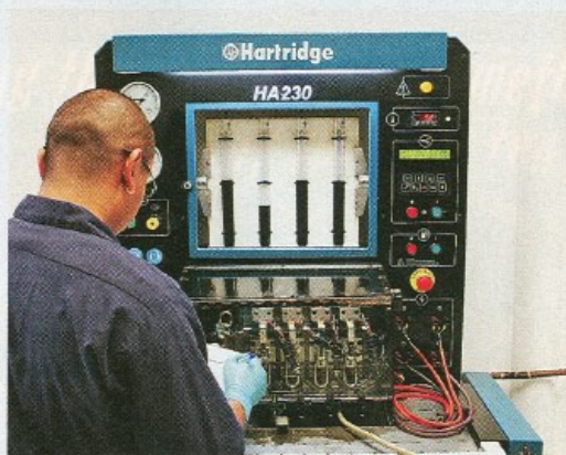
4. The machine fills graduated columns with fuel as they pass through the injectors, indicating flow capacity.
