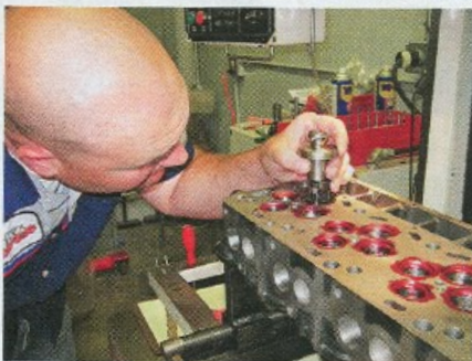
19. The idea is to get a 30-/45-/60-degree transition on the intake valves, or maybe a little better, by keeping a close watch on how much material has been removed and how much remains. Here, the decision is to take off another .005 inch.
