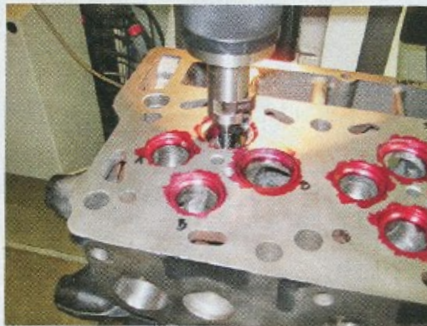
18. The valve seat machining process involves setting up the cutting head to remove a small amount of material, perhaps .005 inch, looking at the result, and then making another cut. The red dye around the valve seats makes it easy to see what has been removed as the process continues.
