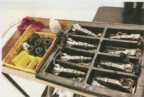
2. Ford injectors used in the 6.0L have a different fuel delivery mechanism from the HUEI injectors used in the earlier 7.3. Instead of using a single solenoid in pulses, the 6.0L fuel delivery is determined by the duration between two open/close commands from the ECU, which actuate magnetic coils on either side of the injector. A piece in between the two coils, called a spool valve, slides back and forth to allow pressurized fuel to enter at precisely metered amounts. If the spool valve becomes contaminated or worn, the injector can't function properly.
