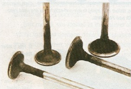
9. The valves were heavily coated with carbon deposits, as well. These deposits may have been the result of contaminated fuel, cold operating conditions, excessive idling or all three.
