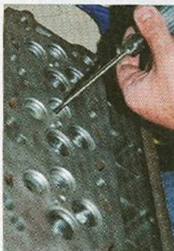
13. The next step is to do a mild port job on the heads to see if airflow can be enhanced. The shape of the valve bowls is probably nearly optimal, but the texture of the casting is definitely rough.
