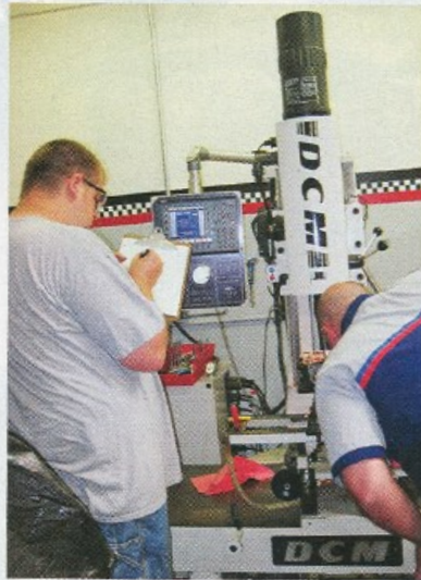
17. After all the ports have been cleaned up, the valves and valve seats need to be machined. After looking at the heads, Banks techs saw that there is not much material on these heads to allow for improvement, something on the order of .020 inches. Still, a careful three-angle valve job should yield a wider valve-to-seat contact patch, and a smoother airflow.
