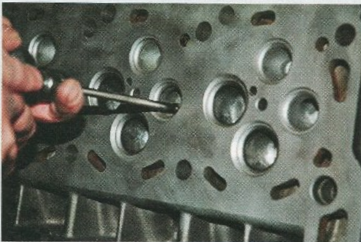
16. On the two smaller exhaust ports, the work was aimed at smoothing out the casting texture and opening up the area under the valve seat in preparation for machining.
