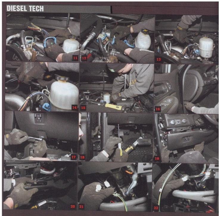
11-12. Insert the factory male connector into the female connector on the SpeedBrake harness and insert the male connector on the SpeedBrake harness into the female connector on the factory harness. Make sure the blue locks are fully seated on both connectors.
