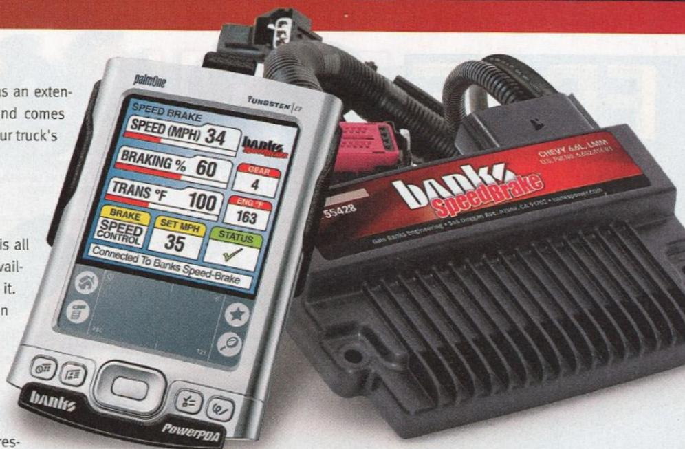
Courtesy of Banks' touch screen PowerPDA, any SpeedBrake feature you want to experience is at your fingertips. The PowerPDA in our test looked similar to the one pictured. We could see which mode the SpeedBrake was in (Speed Control mode with a 35-mph target speed is shown), what braking strength was being applied (60 percent is shown because the target speed was already obtained), transmission temperature, engine coolant temperature, and gear indication.
