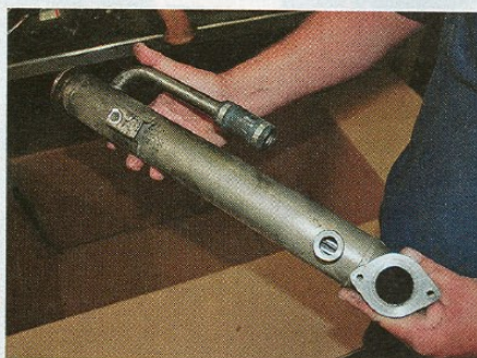
14. The EGR mechanism on early 6.0L engines was a source of a multitude of problems. A Ford service bulletin noted carbon deposits on the EGR valve could lead to turbo vane sticking, plug the MAP sensor hose, and even allow moisture to attack other problems. EGR cooler
