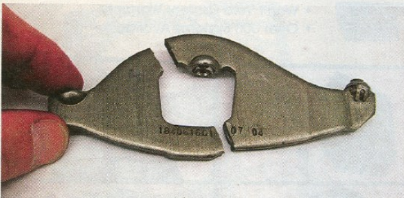
17. Sure enough, the culprit in this particular engine was a rocker that snapped in half. Upon rebuild, all will be replaced with new Ford parts, as no high-performance rockers are available yet for the 6.0.
