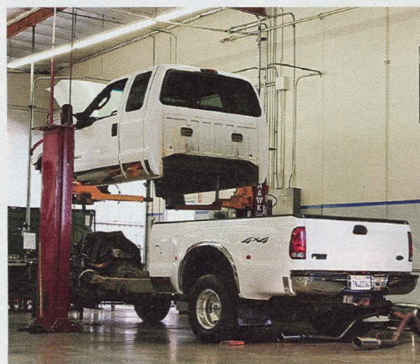
5. To get the cab off the frame involved undoing six rusty body mount bolts, unplugging every connector in sight, and undoing the front brake lines, the throttle cable, ABS plugs, emergency brake cable; removing the exhaust system, oil/transmission cooler lines, fuel lines, steering shaft from the steering box...whew... evacuating the R134 coolant from the A/C system and removing the lines, draining the cooling system and removing the radiator, intercooler and fan shroud...whew...then gingerly moving the body upward slightly to find out what was still attached. Which might include the antilock controller and any of half a dozen plugs that connect the cab to the engine or transmission. The process took an experienced mechanic, working in a highly organized professional environment with power tools and a lift, the better part of a full day.
