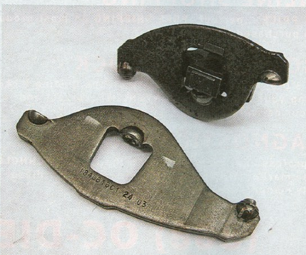
15. A close look at the rocker arms showed some corrosion and slight galling.
