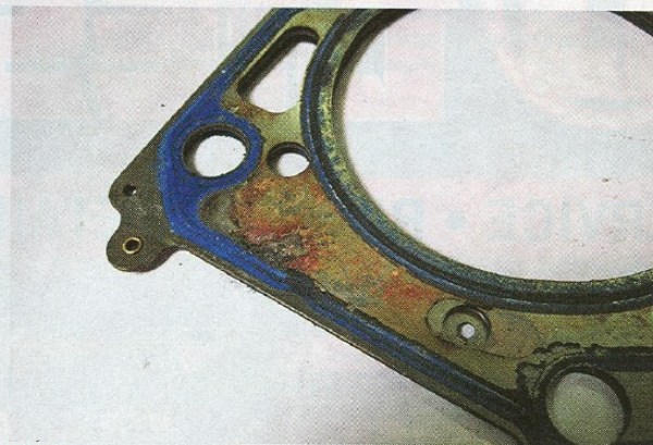
13. There was one portion of the head gasket that had begun to show progress toward leaking, but this gasket never actually gave way.
