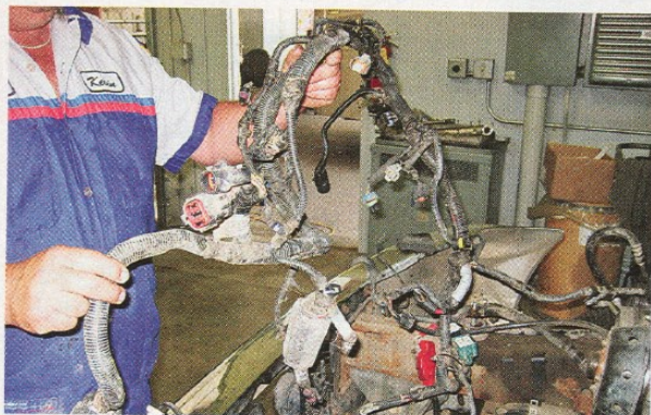
7. Not to put too fine a point on it, but engines these days have just slightly less wiring than the space shuttle. This is the kind of spaghetti you'll be dealing with when you finally get to the engine. Budget another eight hours to remate engine to cab once the rebuild is done.
