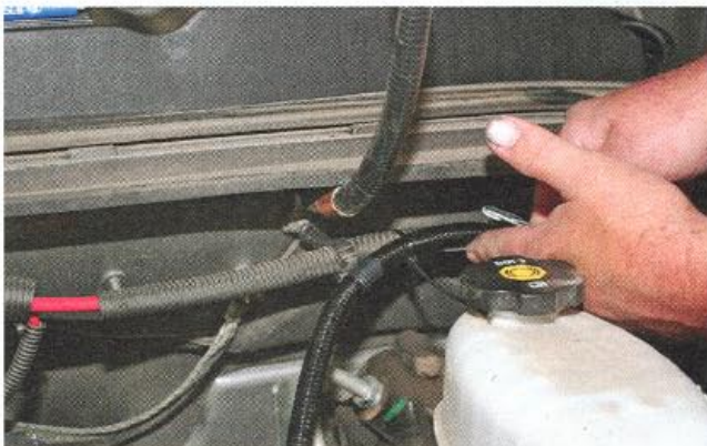
1. Disconnect the negative ground cables from the battery. Locate the SpeedBrake wire harness and start by placing the wire harness near the underhood fuse box. Run the main transmission intercepting connector down to the transmission following the factory main connector harness from the TCM.
