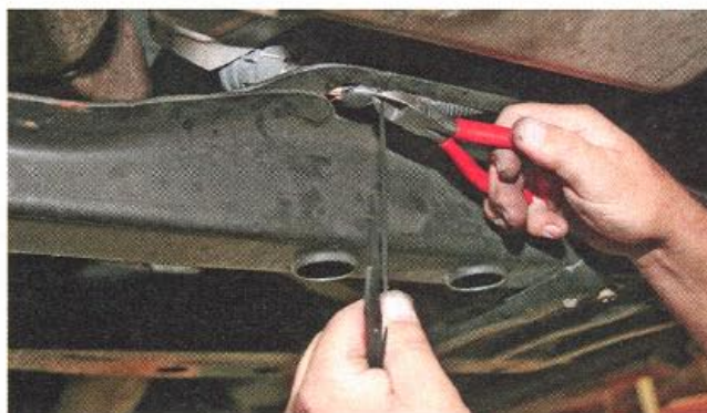
4. Secure the wire harness using some of the supplied cable ties along the factory harness.
