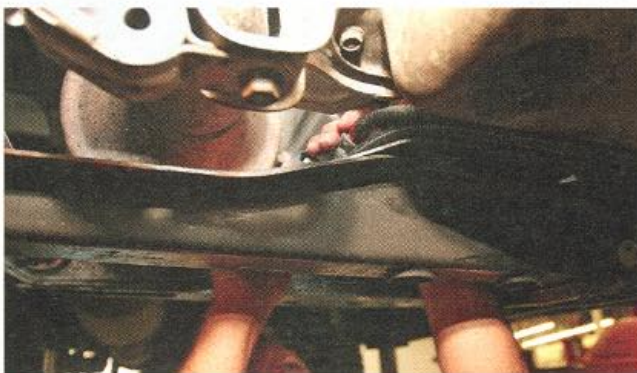
2. The main connector is on the rear right side of the transmission. Disconnect the plug by applying pressure on both sides and pulling out.
