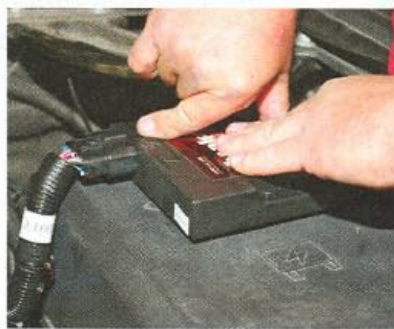
14. Position the SpeedBrake module on top of the fuse box to the edge closest to the engine side of the fuse cover, and then press adhesive onto the outside of the cover.
