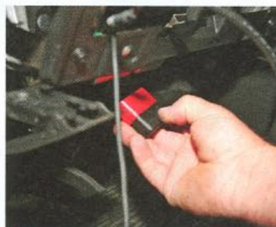
17. Find the Banks OBDII interface cable and secure it to the vehicle's OBDII connector. Connect the 6-terminal plug to the 6-pin connector on the Banks SpeedBrake wire harness.
