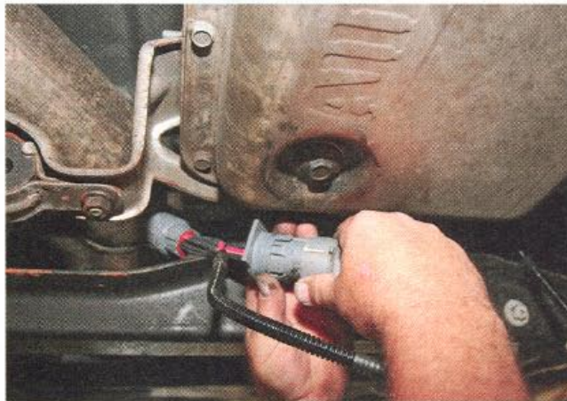
3. Insert the female connector on the SpeedBrake wire harness into the transmission connector, and the male connector on the SpeedBrake wire harness.
