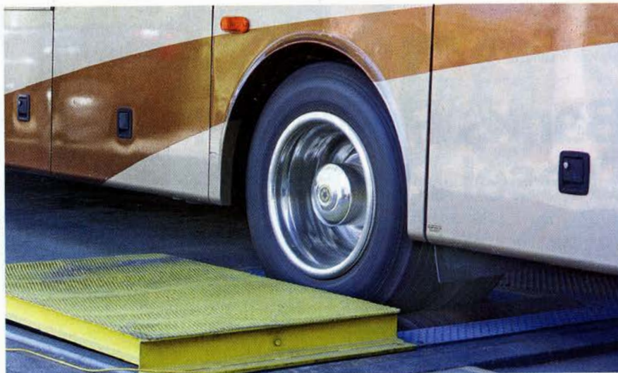
Measuring power at the drive wheels results in real-world numbers directly relating to performance you get on the road.
