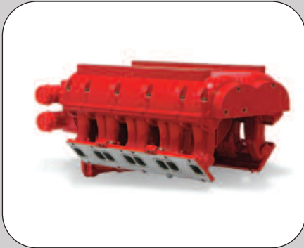
Gale Banks integrated manifold and air-to-water intercooler assembly for DMAX applications. Ram-tuned, tapered runners bolt to the main intercooler body and are CNC port-matched for various Duramax cylinder heads.
