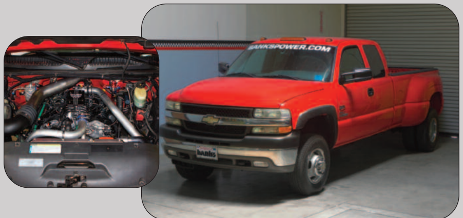
Backwards into the future! A Banks 3.0L 630T V-6 and 6745E six-speed transmission, making 300 hp and 502 lb.-ft., replaces the original 6.6L Duramax with 300 hp and 520 lb.-ft. Performance in this 1-ton dually is identical.
