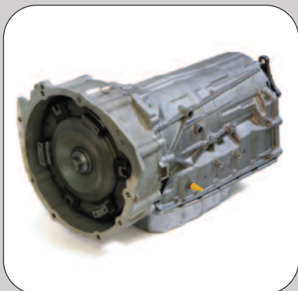
The six-speed Banks 6745E gearbox used with 630T or 866/870T engines. A 300mm twin-clutch torque converter is used.
