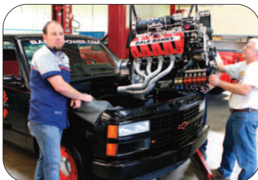
Banks offers swap kits for Duramax into 1987-1998 fourth-gen Chevy and GMC pickups and Suburbans (GMT 400).
