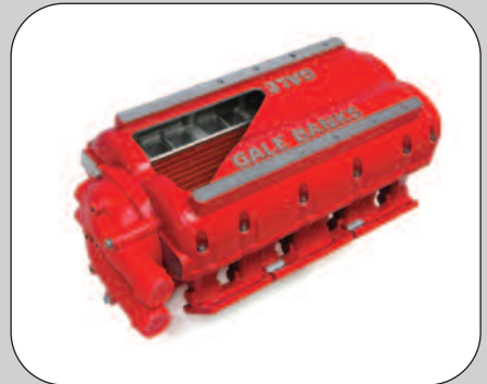
Gale Banks integrated manifold and air-to-water intercooler assembly for Duramax applications. The cut-away intercooler body shows the exit face of the cupro-nickel core and ram-tuned runner inlets.
