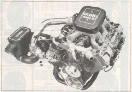
A turbocharger is actually two turbines on a common shaft. Exhaust gasses spin the "hot side" turbine (A) which turns the compressor (B) or "cold side" turbine. The compressor forces more air into the cylinders and a recalibrated injection pump supplies additional fuel. A 3-inch-diameter, low backpressure exhaust system completes the installation.
