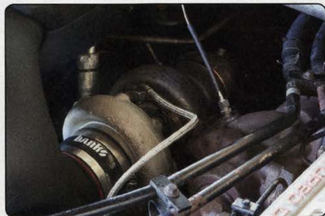
11 For this particular project, a larger, experimental wastegated turbocharger was used to deliver greater air density and reduce EGT, in anticipation of the water-methanol injection. Peak boost more than doubled, going from 16.4 psi stock to 34.4 psi, a gain of 18 psi.
