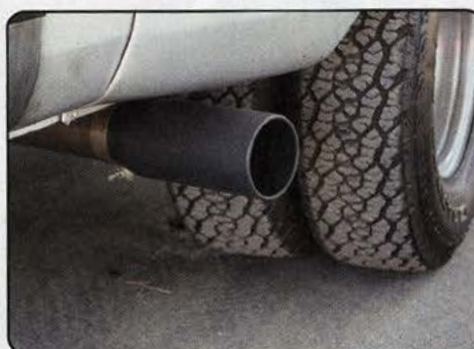
12 The Banks Monster exhaust, which includes both a downpipe and a 4-inch cat-back tube, reduces exhaust backpressure, dropping from 1.6 psi (stock) to .6 psi.
