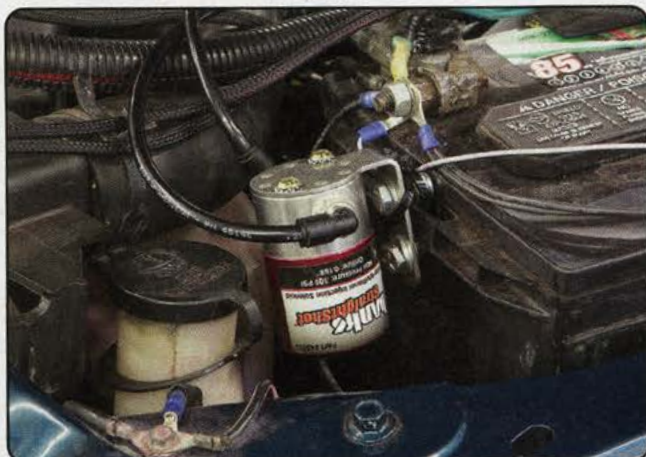
2 The solenoid for the Banks Straight-Shot water/meth system doesn't take up much space, and can be mounted right next to the battery, or wherever else is convenient.
