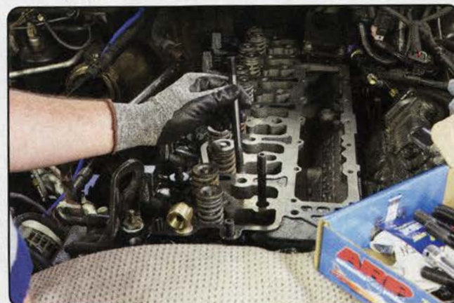
5 The ARP studs are put in only finger tight, so when torque is applied to the nut, the stud will stretch only on the vertical axis. Be sure to apply a generous amount of thread sealer or Loctite to prevent air pockets that might result in leaks. Because the head gasket will compress upon initial torquing, re-torque the bolts after the engine has been run.
