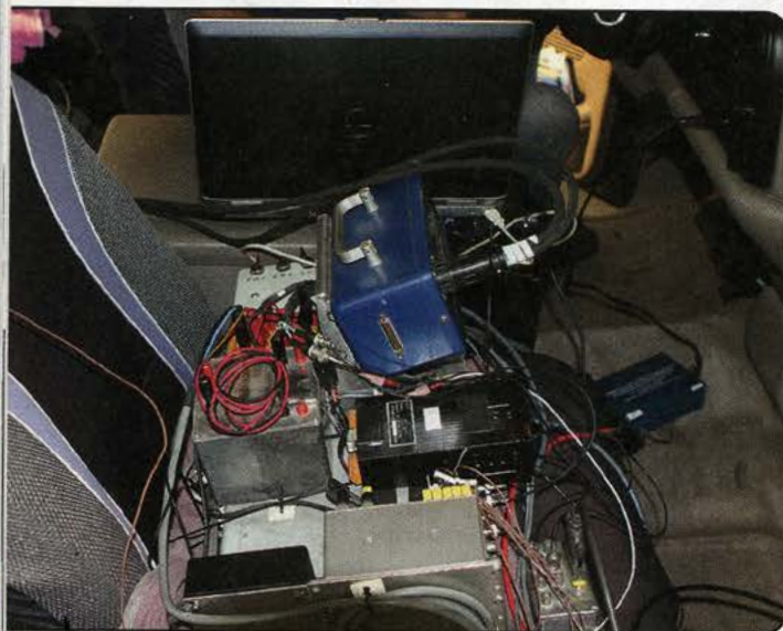
7 This pile of electronics is for data acquisition, along with an opacity meter and tachometer.
