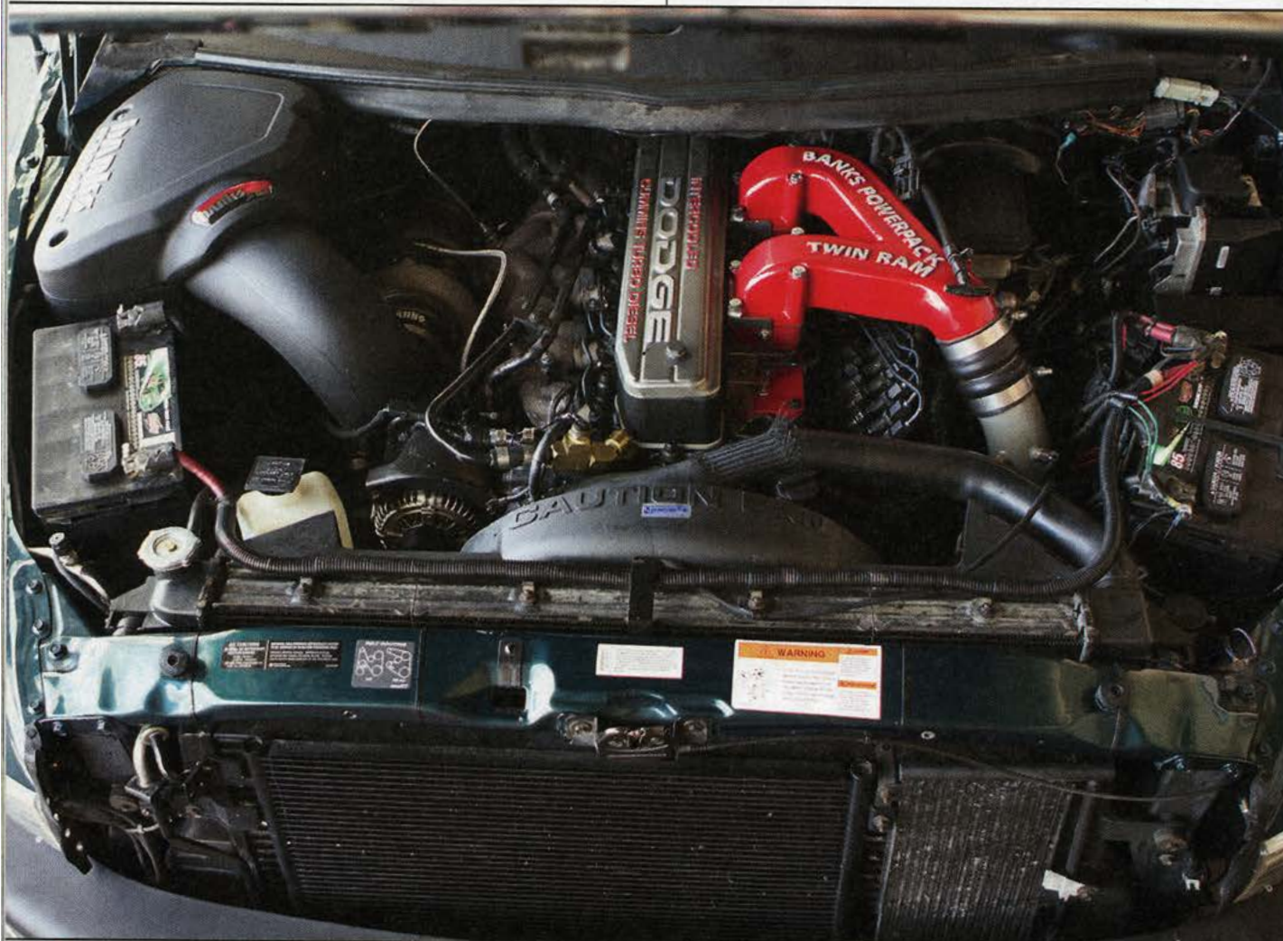
9 Here's the completed install of Banks PowerPack with Double-Shot water/meth system.
