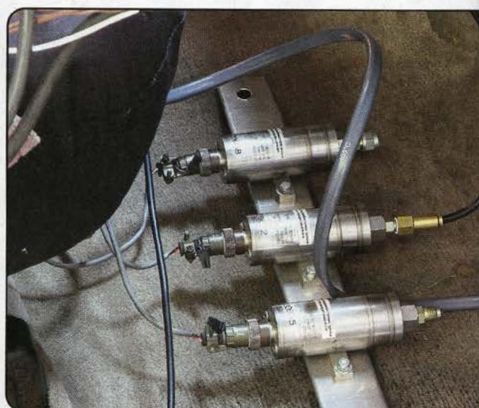
8 These high-accuracy pressure transducers evaluate air density and other variables.
