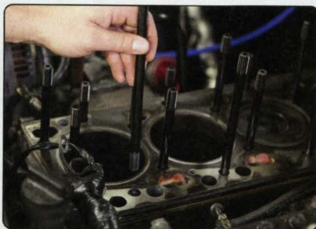
1 After thorough cleaning of the threads, the ARP studs are test fitted and checked for fitment.
