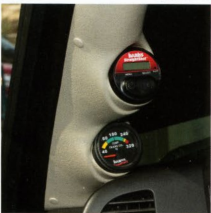
[11] The pillar pod and controller have been set up and all of the wiring is connected.
