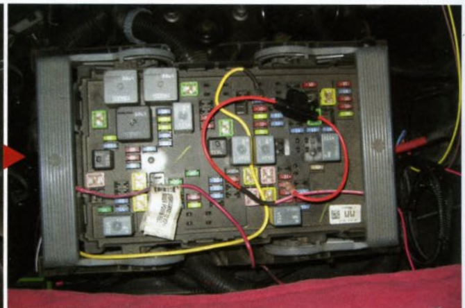
[07] It's best to wire the system up at this point, the harness comes with a fused relay and provisions for a power connector and a tie into the ignition as well.
