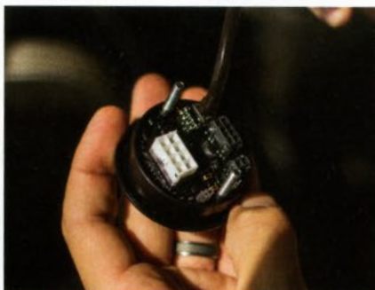
[09] The wiring is run up the pillar and connected to the back of the controller that not only monitors the boost but controls the injection.
