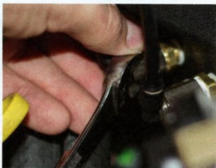
[16] Holes are drilled into the air intake tube in between the supercharger and the throttle body and MAF to avoid any false readings. Then the nozzles are tightened up.
