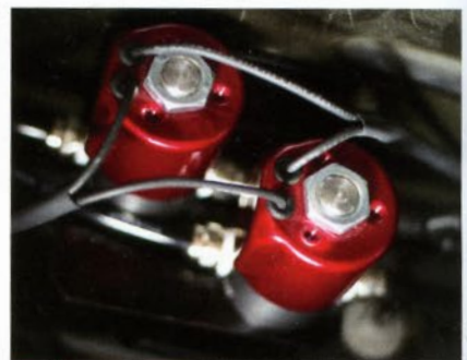
[06] A pair of solenoids that will control the nozzles is installed onto the passenger side inner fender for close proximity to the air intake tube.
