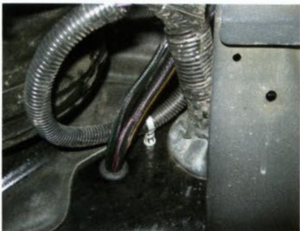
[08] The controller will be mounted in a pod pillar inside of the truck, and the wiring is run through a grommet hole in the firewall. It's best to cover the wires with mesh or loom to prevent damage.
