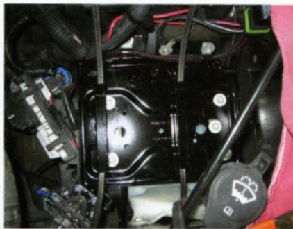
[05] The secondary battery tray is the perfect location to mount the 2 1/2-gallon reservoir tank. It is modified so that the reservoir can be held in place using a pair of straps.
