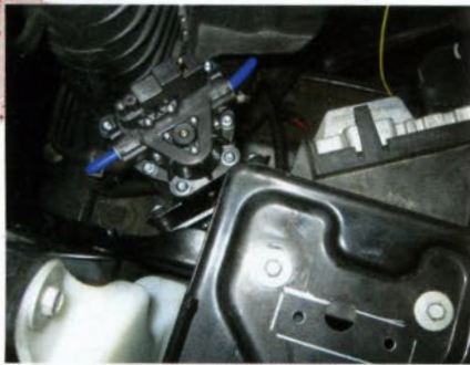
[04] The bracket with pump is installed back into the truck.
