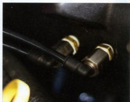
[17] The reason for having two nozzles is so that one can be set to come on at low boost with a low duty cycle and then shut off when the other hits at full duty cycle, with both coming on at full duty cycle at peak boost when needed.
