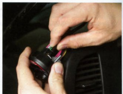
[10] A line ties into the supercharger in order to read boost. You can set up the controller to vary the injection depending on the level of boost. This allows for a more efficient system that only kicks on as needed.
