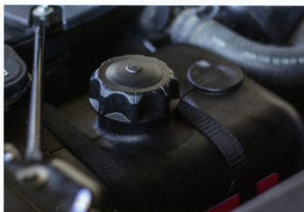
[12] With the wiring finished, the 2 1/2-gallon reservoir is strapped in and connected to both the pump and solenoids.
