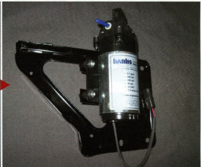
[03] The pump and reservoir are mounted first. The factory ECU bracket that bolts to the inside of the fender is removed and modified in order to mount the Banks Power pump complete with rubber isolators to lessen vibration.
