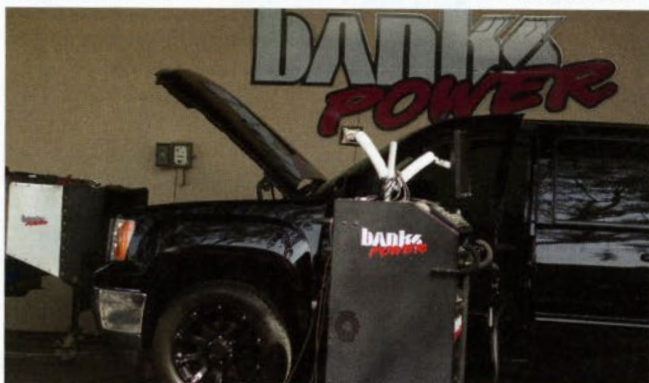
[18] With the system hooked-up and checked, it's time to test it out on the dyno at Banks Power. The true potential of the system is that it safely allows a tuner to maximize the engine with the water-meth injection acting as a safety measure in addition to adding power of its own. HP tuners are used to modify the existing setup in order to change the timing.
