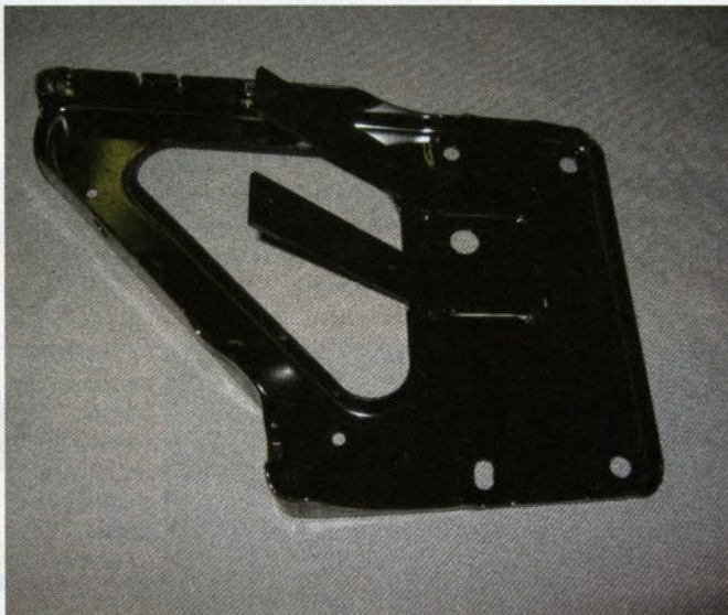
[03] The pump and reservoir are mounted first. The factory ECU bracket that bolts to the inside of the fender is removed and modified in order to mount the Banks Power pump complete with rubber isolators to lessen vibration.
