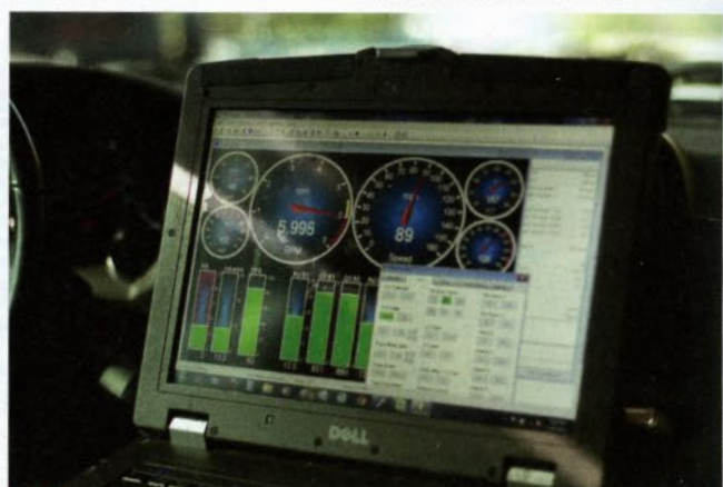
[19] A baseline run with no injection garnered 334 hp and 364 ft-lbs torque. The power was robbed at the top end when the engine hit knock and retarded the timing -4 degrees.
