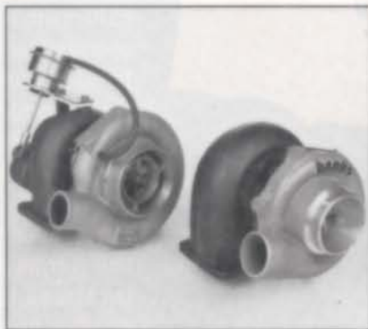
The turbocharger pictured on the left is equipped with a wastegate that limits the maximum boost pressure.
