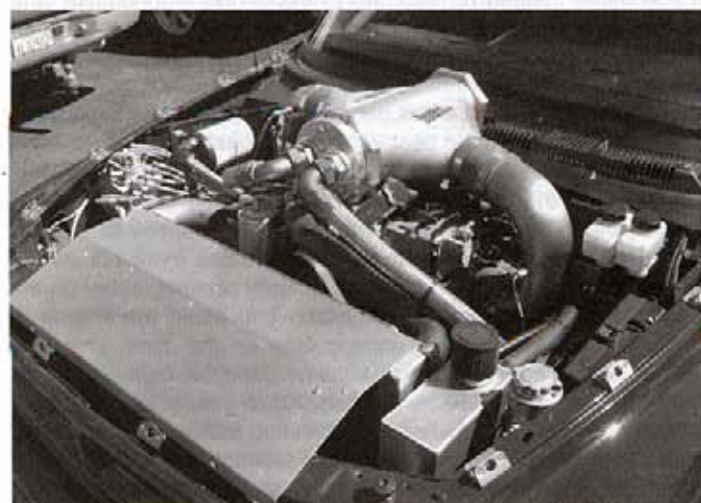
Intercooler atop 5.9 a high-pressure, common-rail Cummins.
