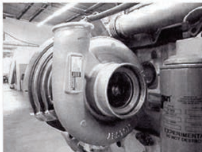
The variable ring nozzle in the Holset HY55 turbocharger must be carefully controlled to prevent unintentional overspeed operation of the turbo. Only electronic controls can respond with the necessary speed.
