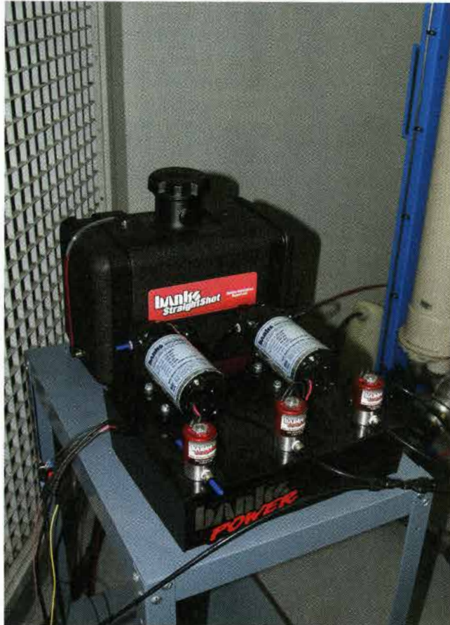
For dyno testing and development, the Banks team pushed the Banks Straight-Shot and Double-Shot systems using this test bed system that used two pumps and three solenoids. It was determined that for production systems, the cost-to-benefit ratio indicated fewer of each would work just fine.
