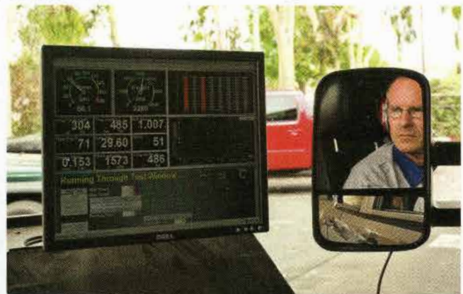
The key to the performance of the Banks water/methanol injection system's smooth operation and great power gains is due to lots of time on the dyno. Small tweaks can mean big gains, but this takes development time and lots of "what-if" testing to get it right.
