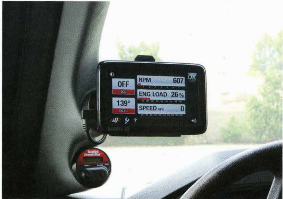
Here you can see the user-adjustable electronic gauge/control unit for the Straight-Shot and Double-Shot systems. It's mounted below the Banks iQ 2.0, another great upgrade for your rig.
